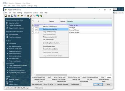
Figure 9: Create a copy of the MIcroShade® glazing you wish to modify.
