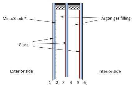
Figure 3: A glazing composition of a 3-layer LowE window with MicroShade<sup>®</sup>. The numbers indicate the indexing of the glazing surfaces.
