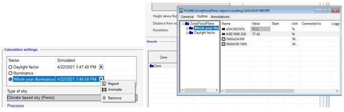
Figure 9: Extract your results as a report or explore the results as an animation through the menu in the upper left corner Figure 10: The results can also be found in the results menu. Note "Whole year illuminance" results only can be found in this menu by double clicking on the zone in the table. Results from the other calculations will be shown in the table.
