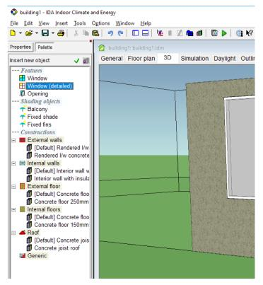
Figure 2: Add a detailed window to the model, by dragging it from the "Palette" menu.
